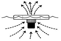
During unit operation, water is circulated from 360° around the unit as well as from below. Top intake for shallow water operation
