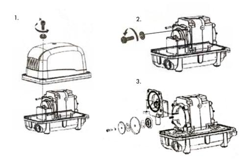
Never operate the unit with defective diaphragms. Always replace the complete pair even if one diaphragm is defective. Failure to follow these instructions can result in electric shock, serious injuries, or even death. Please contact a qualified technician if you did not wish to undertake the replacement yourself.
