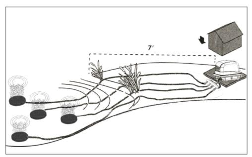
Place the diffuser discs in different locations under water for best aeration results throughout your pond or water source. Weighted tubing will keep discs securely at the bottom of the water. Place each discs no more than 10' under water for best aeration results. See image above.
